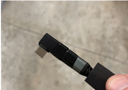
The 90° adapter with a band of electrical tape securing it to the cable.
