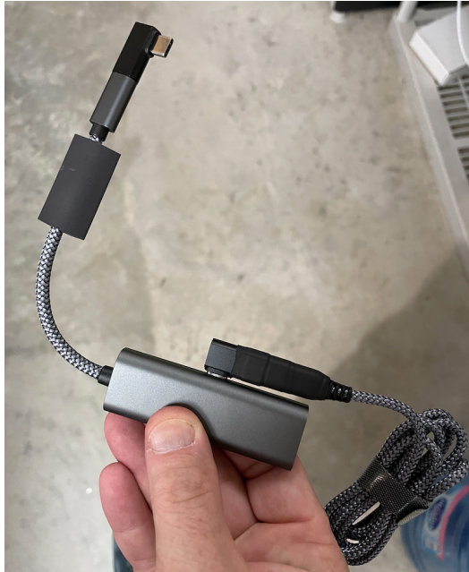
The USB-C to Ethernet adapter with the power input connected and the 90° L adapter.
